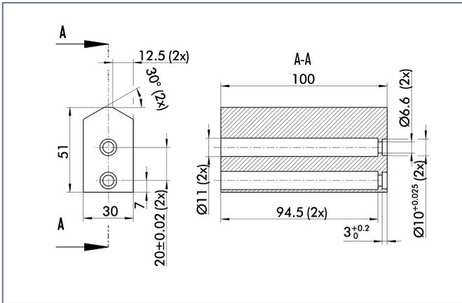
Finger blanks for customized subsequent machining, incl. screw connection diagram.
