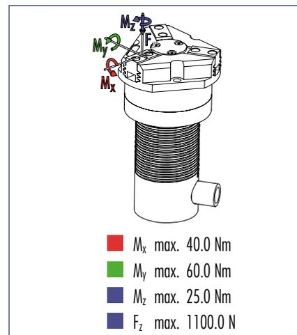
① Moments and forces apply per base jaw and may occur simultaneously.  $M_y$  may arise in addition to the moment generated by the gripping force itself. If the max. permitted finger weight is exceeded, it is imperative to reduce the speed so that the jaw movement occurs without any hitting or bouncing. Tool life may be reduced.
