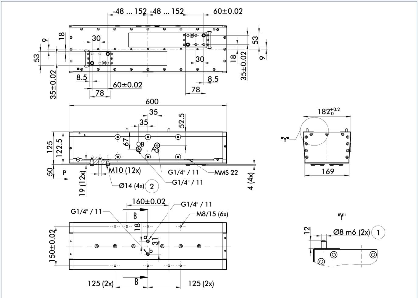
The drawing shows the gripper in the basic version with open jaws, the dimensions do not include the options described below.
