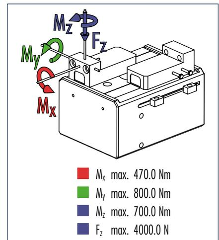
ⓘ Moments and forces apply per base jaw and may occur simultaneously.  $M_y$  may arise in addition to the moment generated by the gripping force itself. If the max. permitted finger weight is exceeded, it is imperative to throttle the air pressure so that the jaw movement occurs without any hitting or bouncing. Service life may be reduced.
