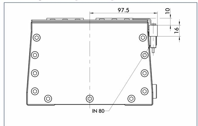
The mounting kit enables 2 inductive proximity switches to be fitted. The kit is fitted in the sensor slot of the slotted switch.
